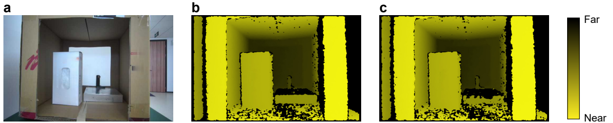
Figure S3: Depth images comparison in a scene without glass. (a) Scene of a cardboard box with its front surface removed. Inside the box, there is a box of gloves and a metal breadboard. (b) Depth image from the PSL 3D sensor, obtained by setting both the TX and RX in TM polarization. (c) Depth image from the PSL 3D sensor, obtained by setting the TX in TM and the RX in TE. The yellow-black color bar applies to both (b) and (c).
